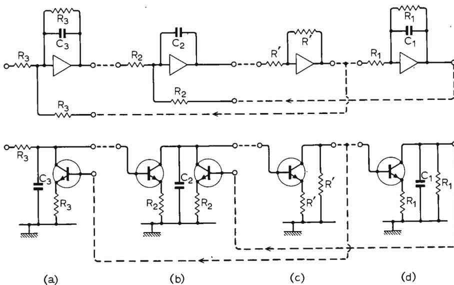
Fig. 14. Replacing the operational amplifiers in a standard leapfrog or active ladder filter by voltage-operated current sources. The constant-current circuits which supply collector current are omitted. As they are in parallel with current sources in the signal path, they should present impedances at least as high.
