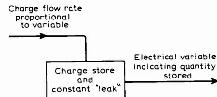
Fig.3. Functional block for a store using electrical charge.
