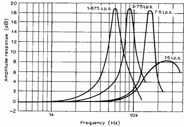
Fig. 6. Frequency response of recording pre-emphasis.
