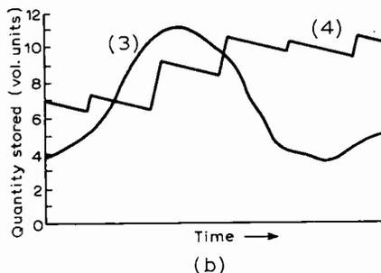
Fig.2. Graphs of quantity stored for Fig.1: (a) with constant inflow; (b) with varying inflow, continuous and pulsating.
