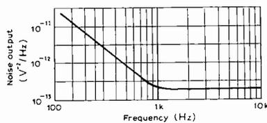
Fig. 9. Output noise spectrum of replay amplifier.
