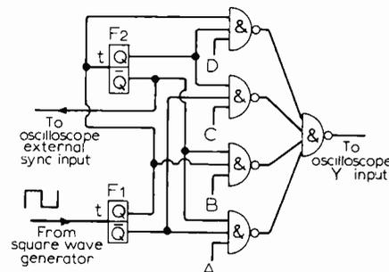
both the circuit under test and the oscilloscope. The oscilloscope's timebase is triggered by one of the flip flops.
