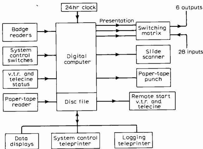
Fig. 5. A process-control digital computer is the heart of this Thames Television system for programme switching and timing.
