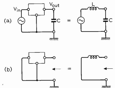
Fig. 17. If the tuning capacitance is removed from a tuned circuit, what is left is an inductance.
