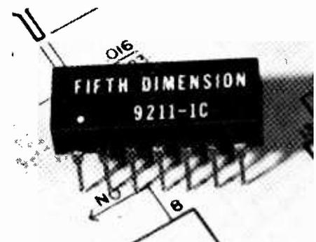
types in the 9000 series—with normally open and changeover contacts, with and without suppression diodes, and monostable and latching types. Made by Fifth Dimension Inc, they are available at prices from about £4 through F.R. Electronics, Wimborne, Dorset BH21 2BJ.
