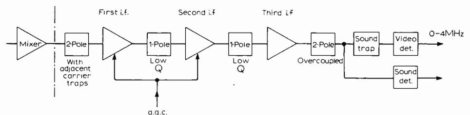
Fig.1. Block diagram of typical transistor i.f. circuitry.
