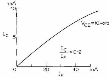
Fig.6. Transfer characteristic of phototransistor/l.e.d.
