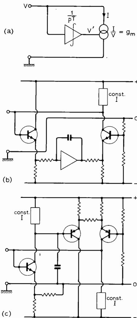
Fig. 3. Inductance-simulating circuits using an integrator and a current source (or mutual conductance).
