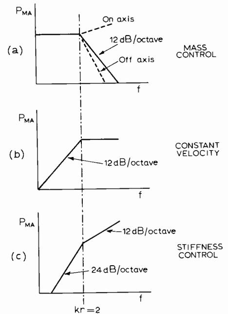
Fig. 5. Effect of mechanical impedance on radiated power assuming a rigid piston in an infinite baffle.
