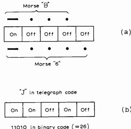
Fig.4. Using on/off patterns in rows of electronic switches for storing (a) Morse characters; (b) telegraph and binary code characters.
