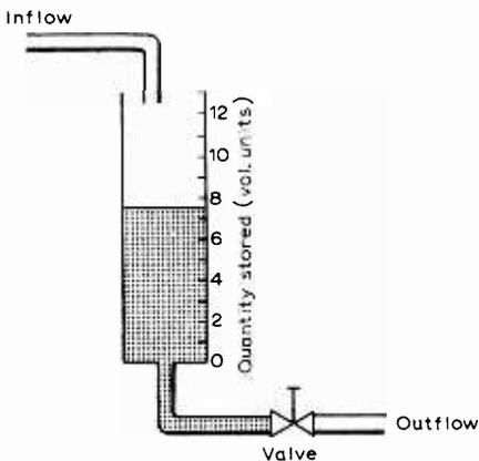
Fig.1. Analogue of a device which stores information by holding electrical charge (quantity of electrons).
