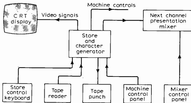
Fig. 4. Automatic programme switching system, controlled by instructions held in a store.
