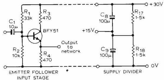
The operational amplifier requires supplies at ±15V, but for a.c.-coupled audio work, the need for a negative supply can be overcome by having a supply at +30V with the input and output of the amplifier held at +15V. Compensation of the amplifier is straightforward, and is achieved by C4 and R11. Pin connections for the amplifier have not been given because they depend on the type of encapsulation.
