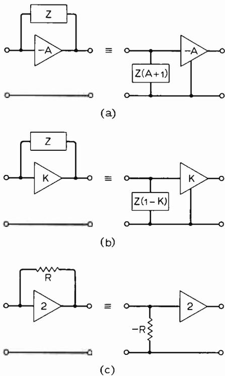
Fig. 10. Equivalent impedances obtained by shunt feedback.
