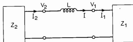
Fig. 16. Two parts of a network joined by a series inductance.
