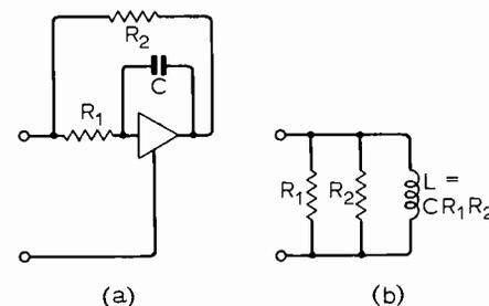
Fig. 7. A low-Q simulated inductance.
