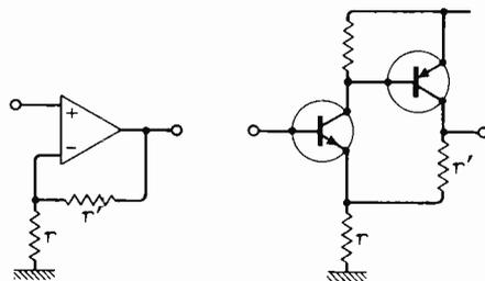
Fig. 12. When internal gain is high, overall gain is determined by the ratio of two resistances.
