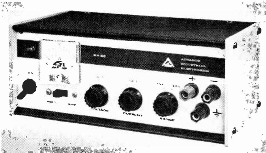
manding applications. Voltage can be set accurately in 10, 1 and 0.1V steps with a digital thumbwheel switch, and down to 0V with a continuously variable fine control. Output current is limited and monitored of course and a variable over-voltage control is provided together with an over-voltage indicator. Two versions give maximum current of 1A (PP41) and 3A (PP42).
