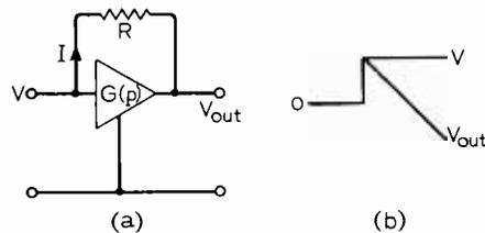
Fig. 5. For  $I = V/pL$  the voltage transfer ratio  $G(p)$  must have the form  $1 - 1/pT$ .
