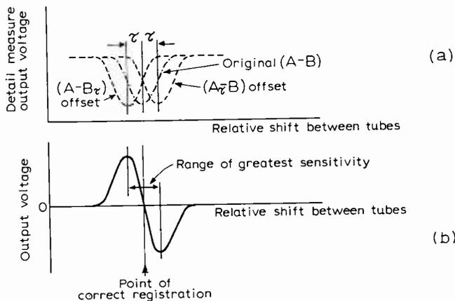
Fig. 1. Principle of system for automatic registration of colour television cameras: (a) two similar responses offset from the original response by delaying signals  $A$  and  $B$ ; (b) output resulting from subtraction of two offset responses in (a).
