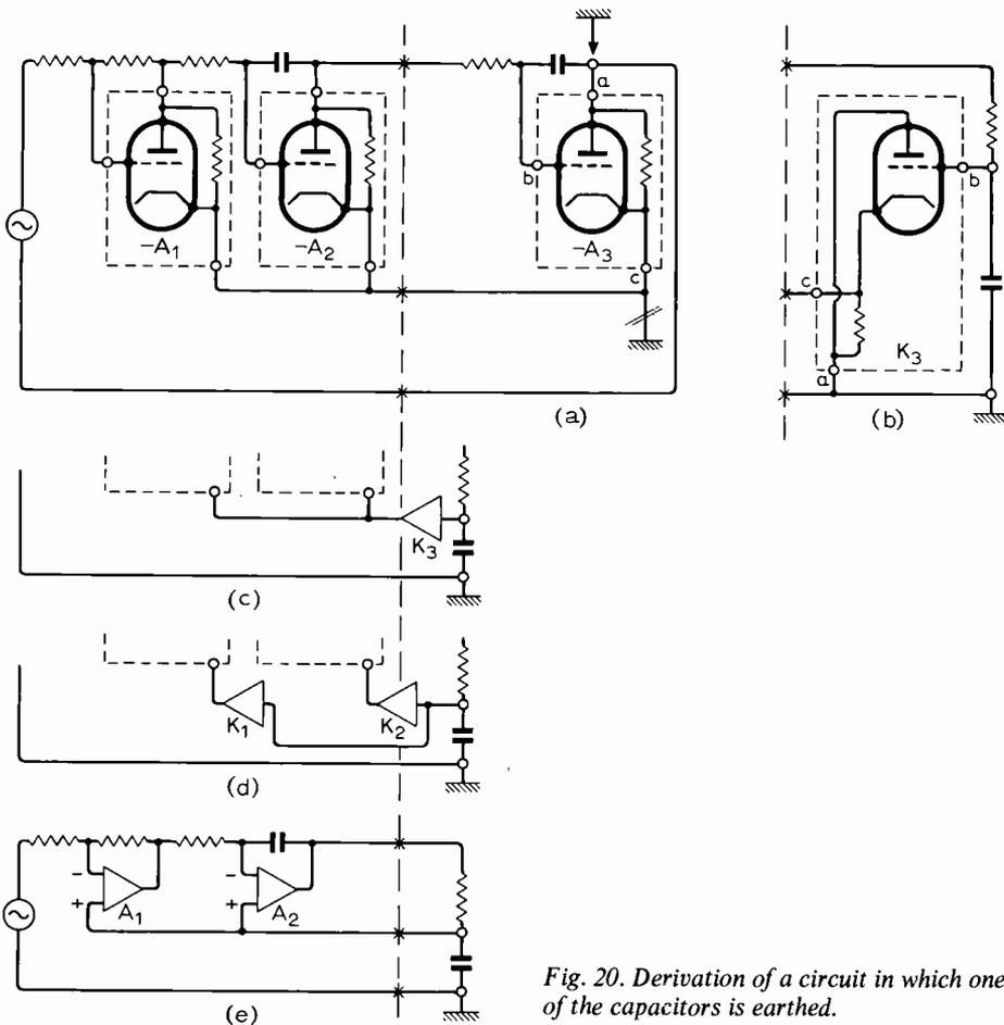
Fig. 20. Derivation of a circuit in which one of the capacitors is earthed.
