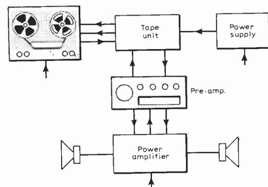
Fig. 2. Expected arrangement of the tape unit.
