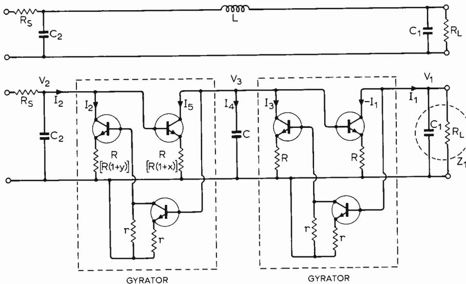
Fig. 15. A method of simulating an unearthed inductance.
