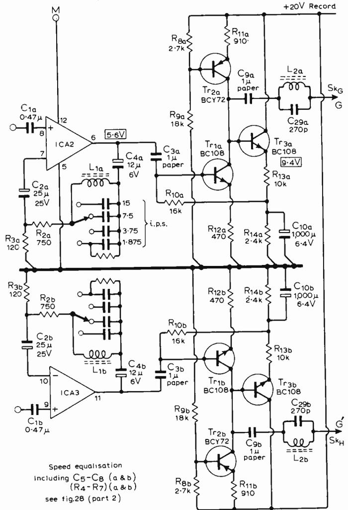
Fig. 5. Circuit diagram of recording stage.
