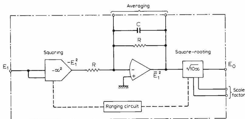
Fig.8. Block diagram of Burr-Brown r.m.s. meter module.
